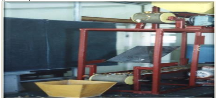
Fig. 1. General view of a device for sorting food waste.
