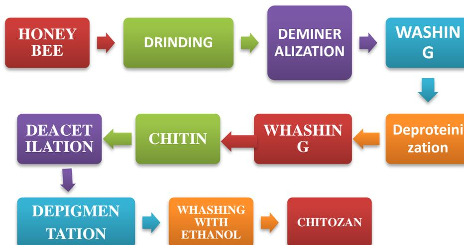
Figure 5. The scheme laboratory technology obtained of Chitin and chitosan from Honey Bee
