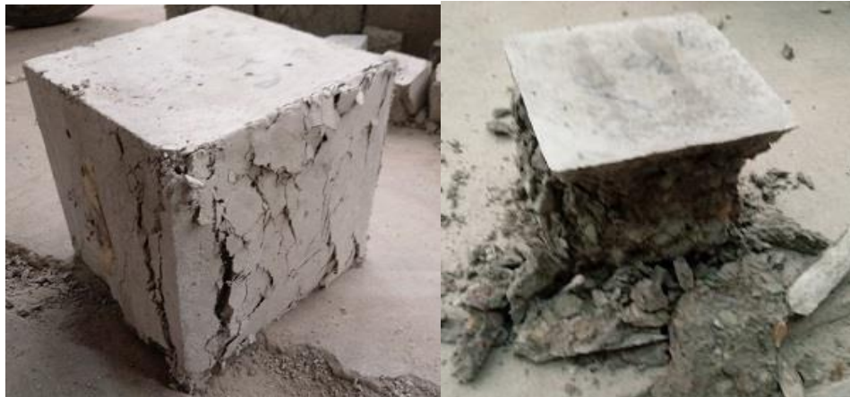
a) Failure of fiber-containing cubic concrete b) Failure of non-fiber cubic concrete
