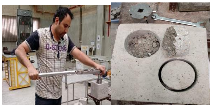
a) Applying bending moment with torque-meter b) Final result of test Figure 1- Friction-transfer test
