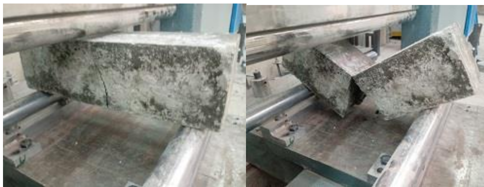
a) Failure of fiber-containing concrete beam sample b) Failure of non-fiber concrete beam sample
