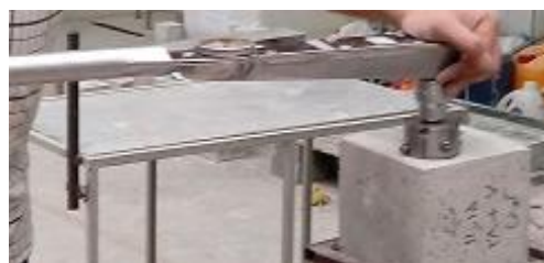
Figure (3): performing the friction-transfer test
