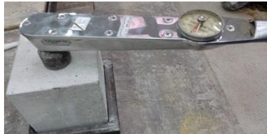
Figure (2): in-situ twist-off test
