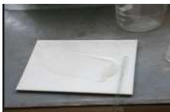
Figure 5. Strontium aluminate is mixed with sodium silicate gel applied on a tile
