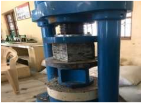
Figure 5. Compressive testing machine and Specimen
