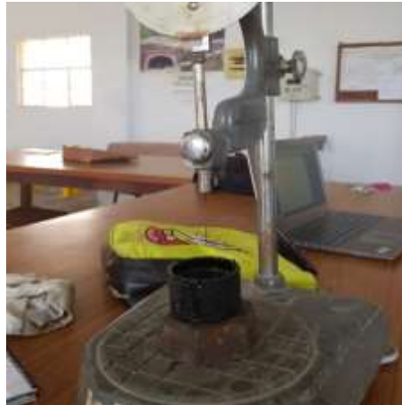
Figure2: Penetration Test in the Laboratory into the Bitumen Mix
