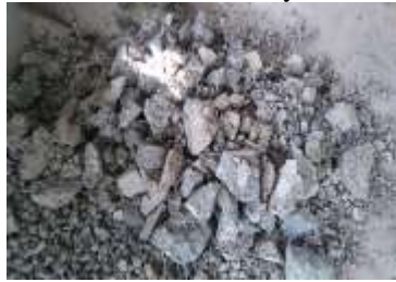
Fig: 2.1 Demolished Concrete Waste
