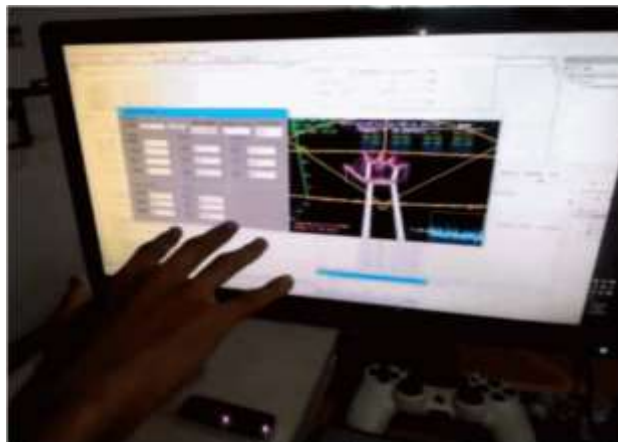
Figure 2: Hand Gestures Tracking System for Browser using Handtrack.js
