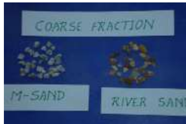
Figure 1. Texture of Coarse Fraction of River Sand and M-Sand Particles
