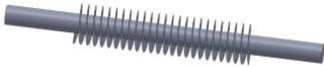
Figure 4: Spiral fin around tube
