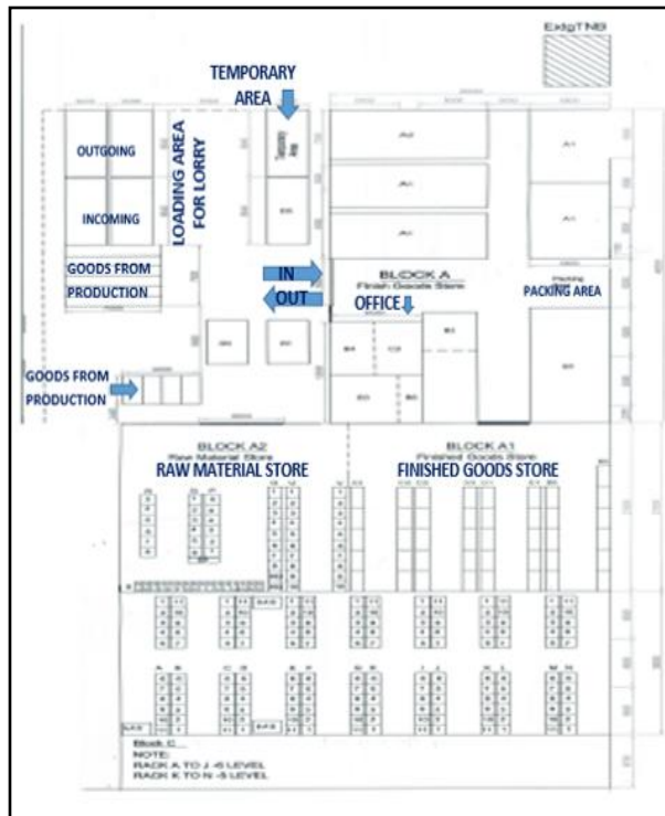
Figure 5. Layout of warehouse TECO
