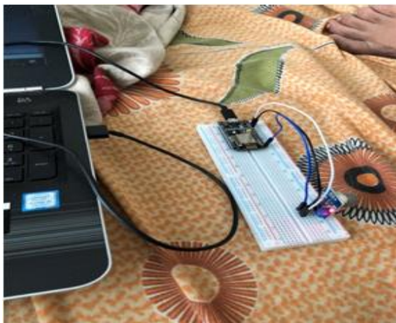
Figure 4.1. Shows the hardware used to detect gas and smoke levels in industries using NodeMCU
