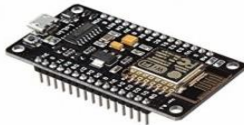
Figure 3.3. Represents NODEMCU - ESP8266 Wi-Fi Development Board
