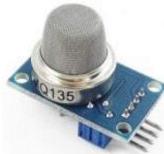
Figure 3.1. Represents MQ135 - Air Quality gas sensor
