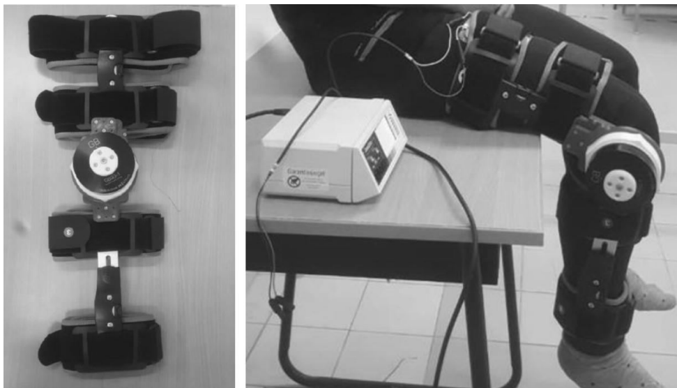
Fig. 5. A developed PKO device with gearbox [76]
