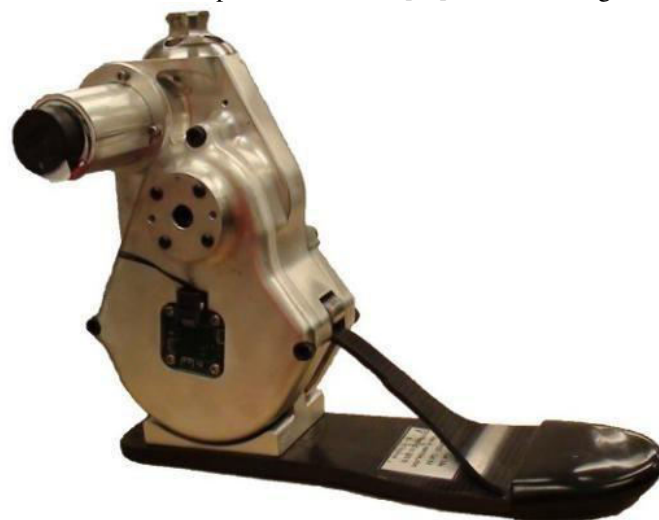
Fig. 3. Vanderbilt Transtibial Prosthesis model [59]
