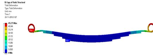
**Figure 11** Deformations in steel
