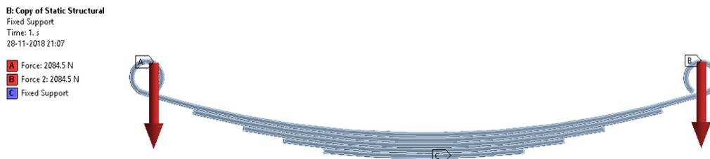
**Figure 4** Structure of leaf spring
