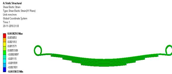
**Figure 9** Shear Strain in E Glass/Epoxy
