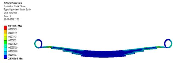
**Figure 6** Strain in E Glass/Epoxy
