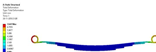
**Figure 5**Deformations in E Glass/Epoxy
