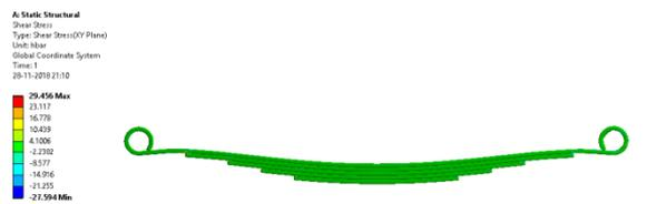
**Figure 10** Shear Stress in E Glass/Epoxy
