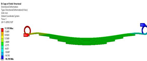
**Figure 14** Directional deformations in steel
