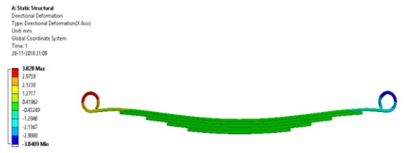
**Figure 8** Directional deformations in E Glass/Epoxy
