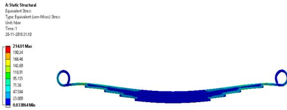
**Figure 7** Stress in E Glass/Epoxy
