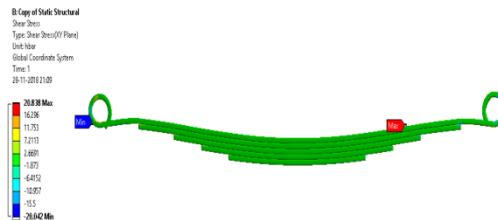
**Figure 16** Shear Stress in steel
