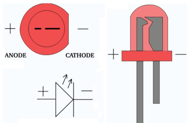
**Fig 2.3.3: Electrical Symbol & Polarities of LED**
