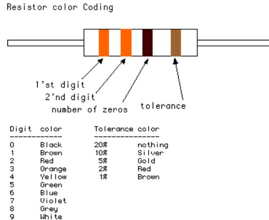
**Fig2.4.2 : Color Bands In Resistor**
