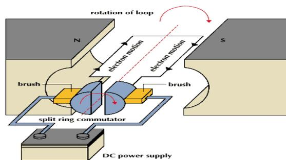
**Fig 2.6.2: Operation of a DC Motor**
