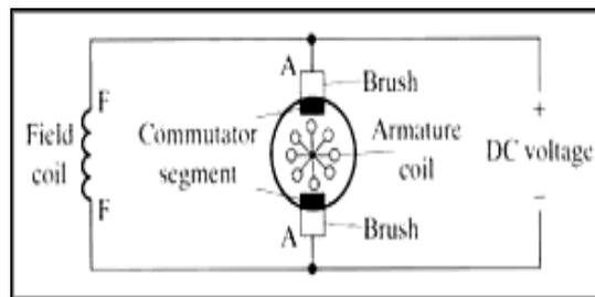
**Fig : Simple electrical diagram of DC motor**
