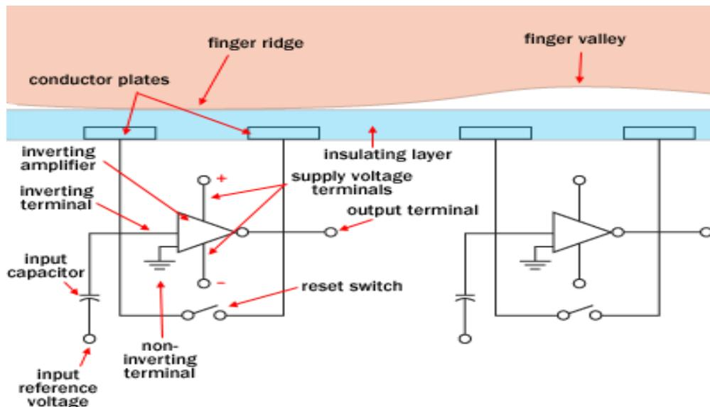
When the finger is placed for recognition, it acts as another capacitor plate. It is separated with
