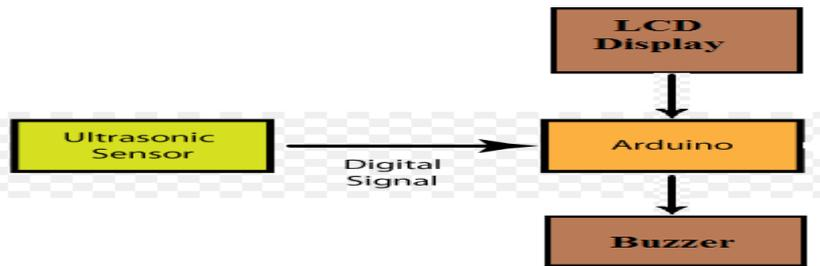
The echo time response of ultrasonic sensor detector is based on time of travel after trigger pulse to the surrounding objects is non-linear and depends on the reflectance characteristics of the object surface.
