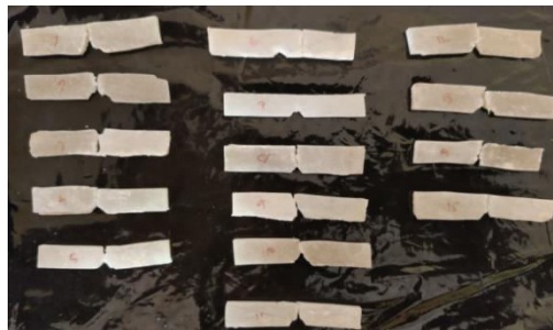
Fig 5: Samples After Impact Test
