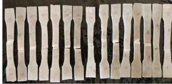
Fig 7: Samples After Tensile Test
