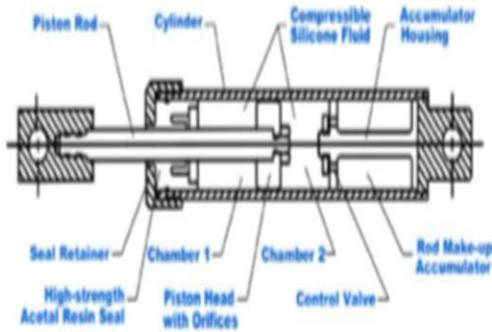
Fig: 1.2 Typical Representation of Fluid Viscous Damper
