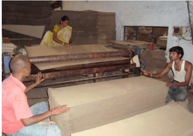
Then these card boards are transferred to creasing and cutting machine where extra material is removed and creasing operation is performed(i.e., from where the box get folded).
