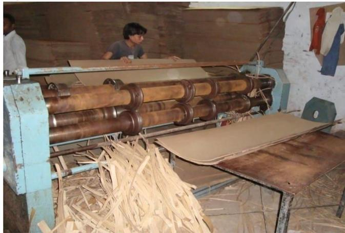
The next operation is slotting operation and finally with stitching operation corrugated box is manufactured.
