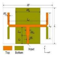
To achieve an Omni directional radiation pattern, an array of such a Quadra pole antenna must be arranged along the current flow direction on dipoles. However, to feed it, we need to use a proper feed network.
