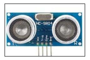
VCC – 5V, input power TRIG – Trigger Input
