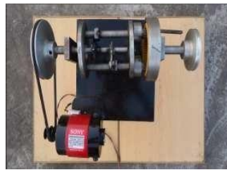
Fig 6 Fabricated Eclipse Gear Box Model With Two Linkages
