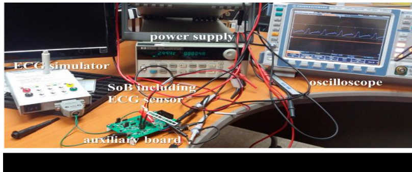
Figure7 Power consumption test for ECG sensor
