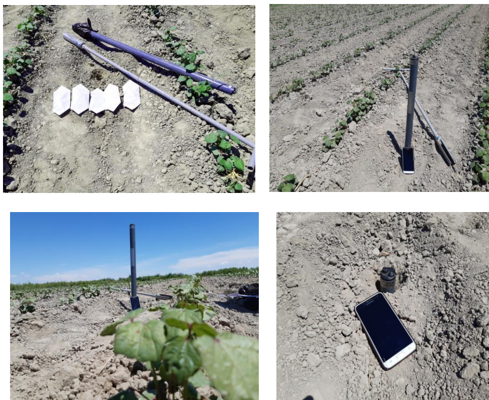
Picture 5. The process of conducting soil analysis through UMP-1 measurement device
