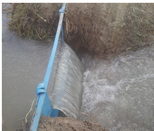
Picture 3. Water flow measurement with using Chipoletti-75 water droplet
