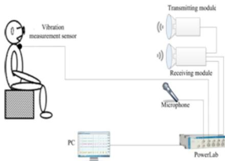
**Fig. 1: Measurement of Vibration in the Vocal Track Using RADAR**
