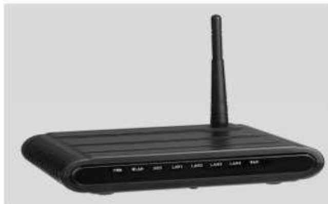
Figure 1: Access Point of Wi-Fi
