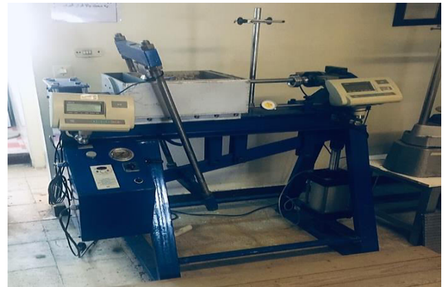
Figure 2 Direct-shear test device
