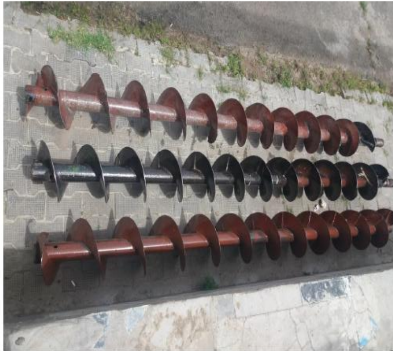
FIGURE 1. Helical conveyors of cotton seeds coated with heterocomposite coatings subjected to solar treatment. Dispersion analysis of mineral fillers was performed on a device of a particle size analysis system in the laboratory of Angren Kaolin LLC on a SediGraph 5100 instrument from MICRO MERITICSINSTRUMENTCORPORATION.
