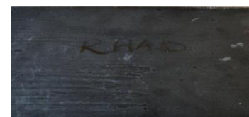
45wt% epoxy+50% glass fiber+5wt% Rice Husk Ash
