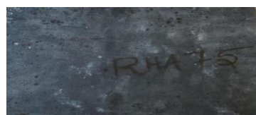
42.5wt% epoxy +50wt% glass fiber +7.5wt%Rice Husk Ash
