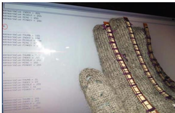
Fig.9: Gesture for the letter B and its corresponding text is displayed
