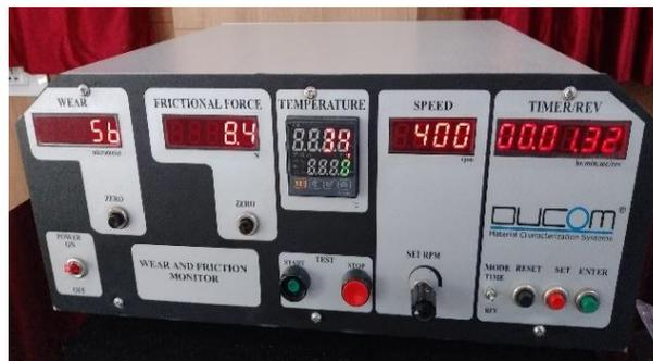
**Figure 7 Control Unit of Pin on Disc Apparatus**
