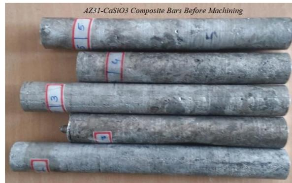
**Fig- 2 AZ31-CaSiO<sub>3</sub> Composite Bars before Machining**
