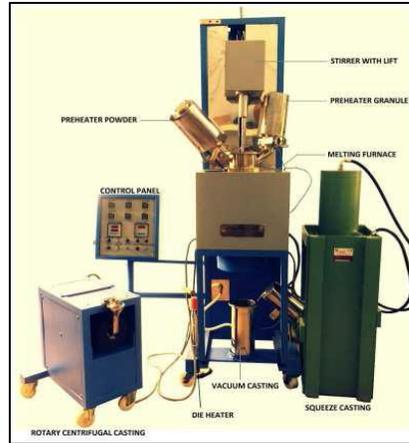
**Fig- 1 Bottom Pouring Type Stir Casting Furnace (Received authorised certificate by corresponding author from M/s. Swam Equip, Chennai, India for using their furnace)**
