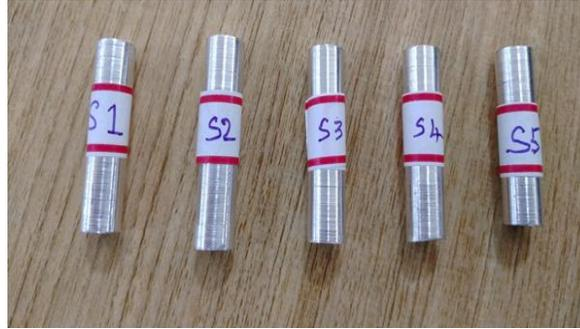
Fig- 4 AZ31-CaSiO<sub>3</sub> Composite Samples for Wear test
