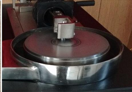
**Fig- 6 Pin on Disc Apparatus**
