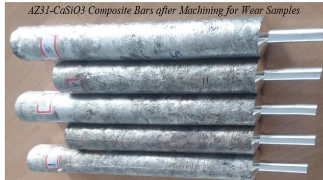
**Fig- 3 Machined AZ31-CaSiO<sub>3</sub> Composite Bars for wear test**
