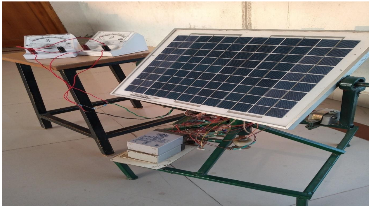
Figure 5. Experimental setup of two-dimensional solar panel rotation circuit for optimizing power generation.
