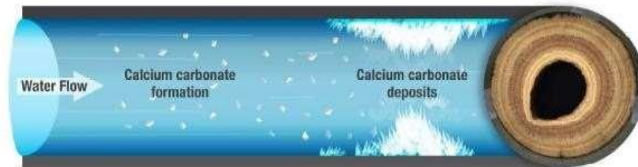
Fig: (3.4) scale formation inside pipe
