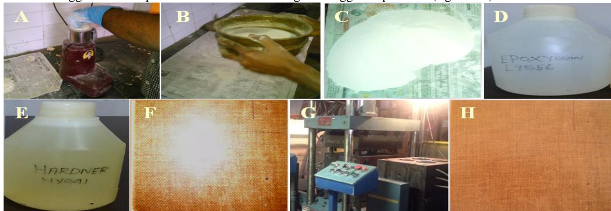
Figure 1. (A) Egg shell’s grinding process (B) Grinded egg shell powder separation process (C) Grinded and filtered egg shell powder (D) Epoxy resin – LY556 (E) Hardner – HY991 (F) Jute fiber mate (G) Compression moulding machine (H) Jute fiber/Epoxy Resin/Egg shell composite plate
