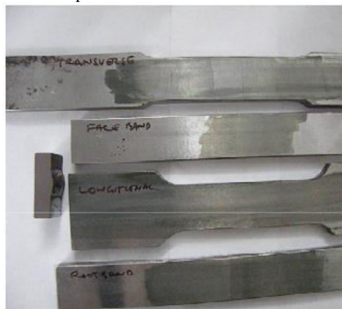
Testing Samples of Base Material before Tensile, Yield Testing and Face and Bend Root Tests
