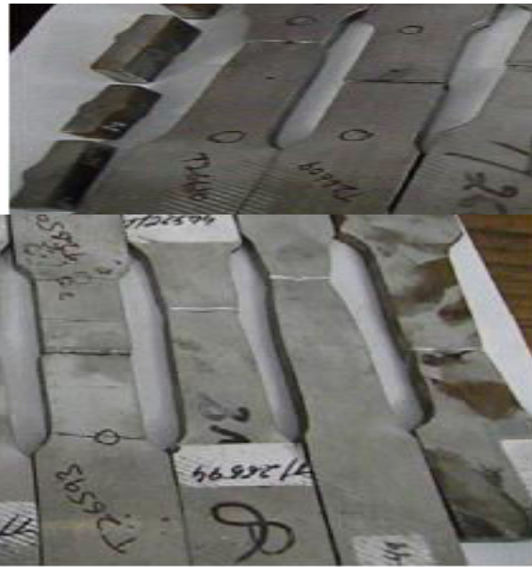
Broken Test Samples after Yield, Tensile and Bend Tests
