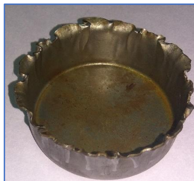
Figure 11: The successful deep drawn cup
