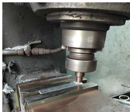
Fig 1. Vertical Lathe Machine During FSP
