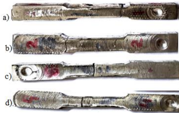
Fig 3. After tensile test specimens a) AZ91D b) AZ91D +2%ZrO 2 +3%B 4 C c) AZ91D + 2%ZrO 2 +5%B 4 C d) AZ91D + 2%ZrO 2 +7%B 4 C
