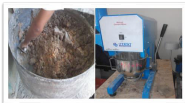
Figure .1. Manual and electric mixing
