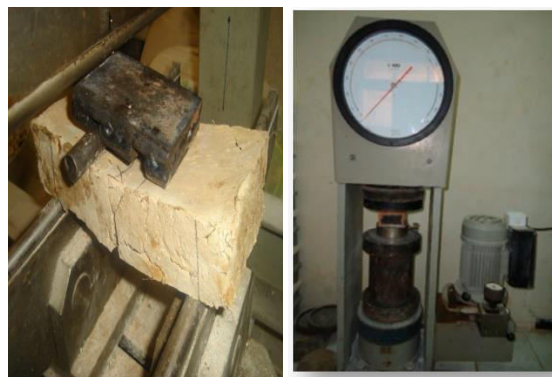
Figure .3 Four-point flexure test and Simple Compression Experience
