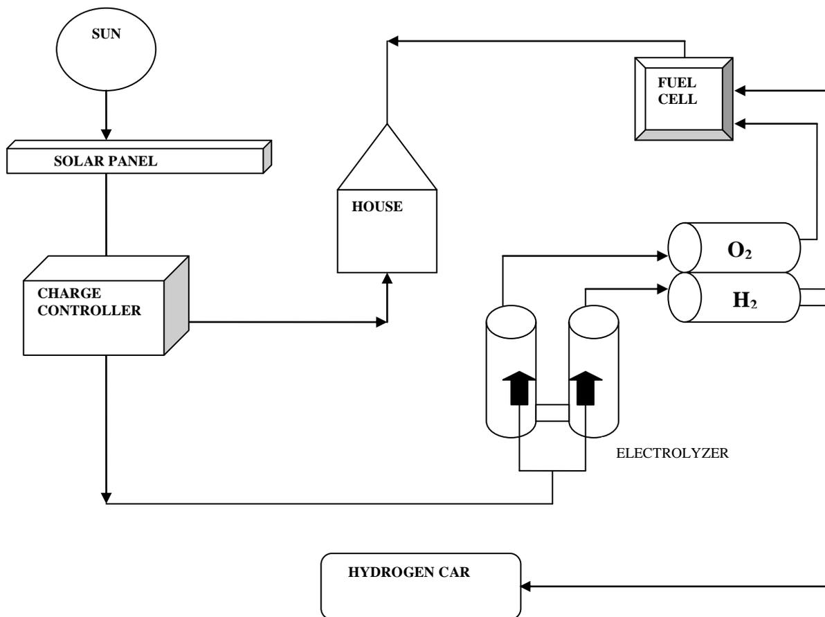
Fig 1. Concept of solar hydrogen house
