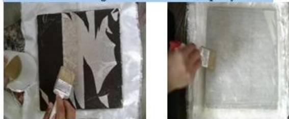
Figure 4 depicts the process of attaching the Glass Fabric to the Core.
