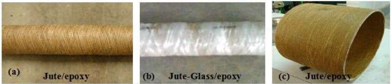
Figure 2. Pipes fabricated, (a) and (b) Using filament winding machine, (c) Using lathe.
