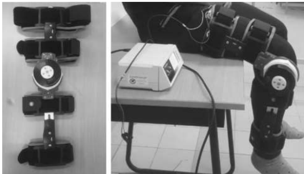
Fig. 5. A developed PKO device with gearbox [76]
