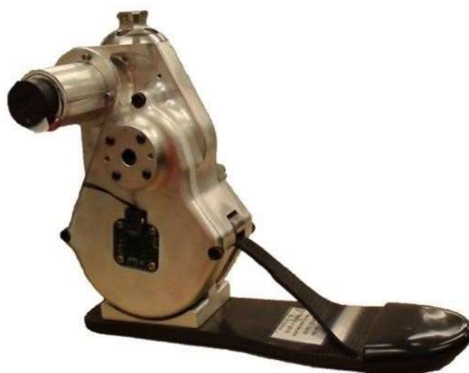
Fig. 3. Vanderbilt Transtibial Prosthesis model [59]
