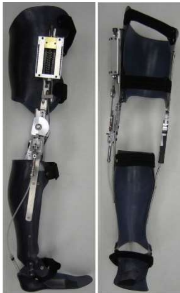
Fig. 4. KEA prototype mounted on a standard KAFO with articulating ankle joints [65]
