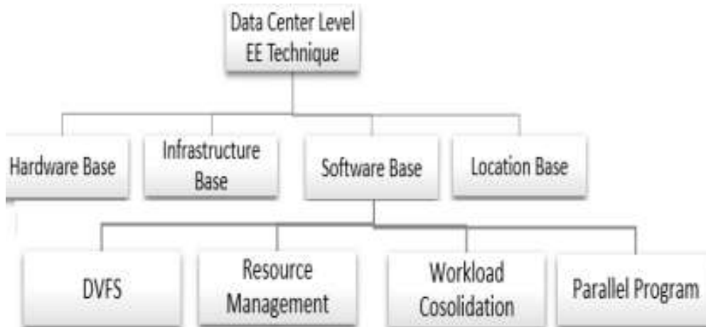
Figure 2: Energy Optimization Techniques at Data Center Level
