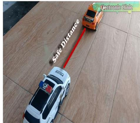
The underlying stage starts from ultrasonic sensor that recognizes the separation of vehicle in the front. If the vehicle arrives at nearer to front vehicle, red shading light will shine that will show warning.
