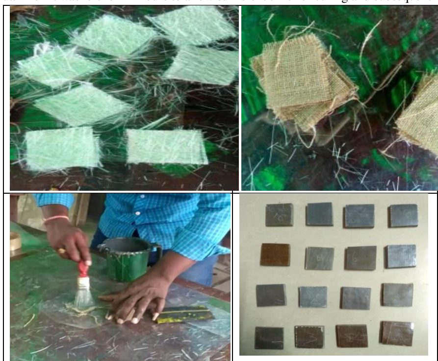
Fig.4 Hand Lay-up techniques of Hybrid composites
