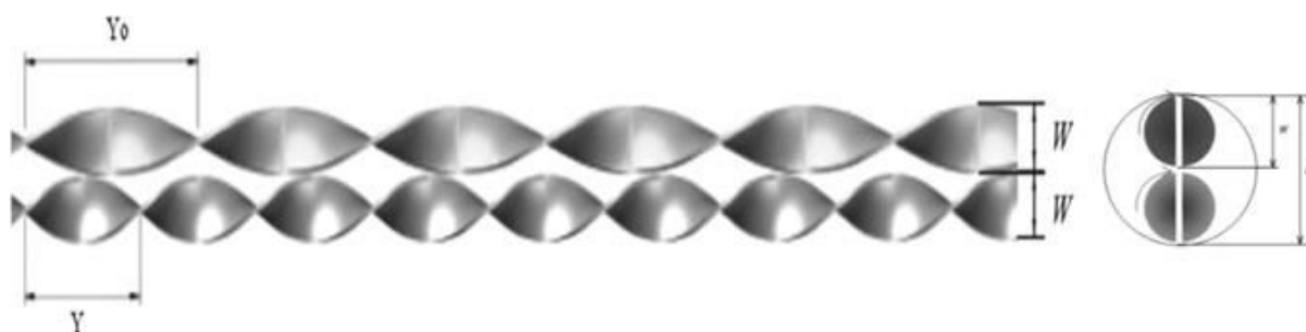
Fig. 2.1 Overlapped dual twisted tapes (ODTTs) and its nomenclature
