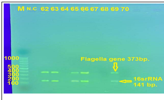
Figure (2): Agarose gel electrophoresis analysis 1% (stained with safe stain) of PCR products presenting gene amplified with specific primers that showed the expected size 141 bp For 16SrRNA and 373 bp for Flagella protein. Lane M: is 100 bp DNA Marker; Lane 2 negative control; Lanes 3-11: gene product amplified from H. pylori genome run on 85V for 45min including samples from 62 to 70. Samples number 62, 63, 65, 66 and 69 showed positive results for both Flag. Protein and 16SrRNA, other samples, 64, 67, 68 and 70 were negative for both Flag and 16SrRNA.
