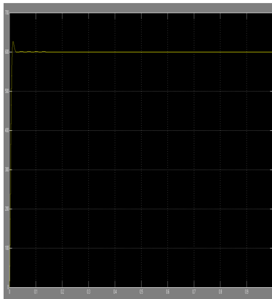
Fig. 6: DC-link voltage for the proposed front-end converter under load variations
