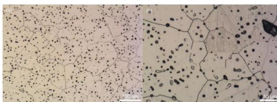
**Figure 5. Microstructure of 316L stainless steel sintered at 5 °C/min (a)with the detail of deformation-induced martensite (b).**
