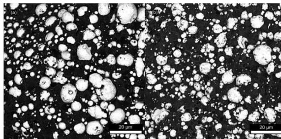
**Fig. 1: SEM micrograph of: (a) acrawax (AW) based feedstock; (b) carnauba wax (CW) based feedstock.**
