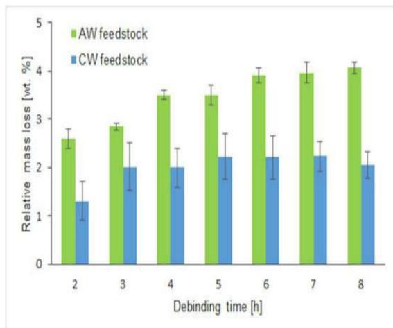
**Figure 3. Relative mass loss during water debinding of CW- and AW-based feedstocks**
