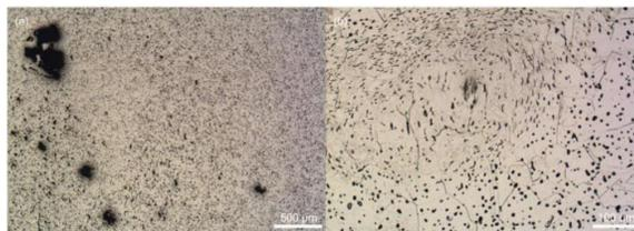
**Figure 6. Microstructures of 316L stainless steel: (a) large defects on sintered area for 10 °C/min speed; (b) vortexes located around larger pores at 15 °C/min speed.**
